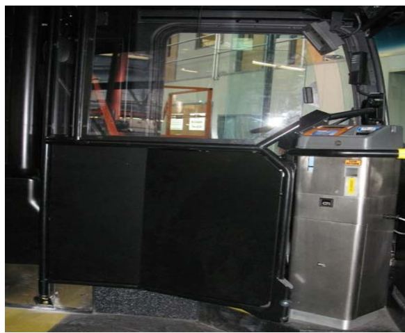
Every coach in the fleet is equipped with a drivers barrier
